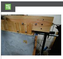
To understand the motion of each member of the specimen, a motion capture system was used.
