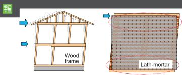
In case of an earthquake, a large relative displacement between the lath-mortar and the wood frame occurs.
