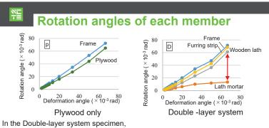
the lath-mortar's rotation angle was relatively small due to the orthogonal wall. The staples fastening the lath-mortar to the wooden lath withdrew or broke.
